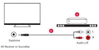
**Note:** The output audio level is dependent upon the headphone level. The volume level on the connected audio system must be turned up.
