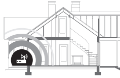
Unsuitable router position
