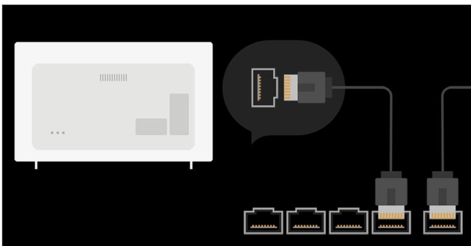
01 Connect the LAN port of the TV and the router using a LAN cable.
