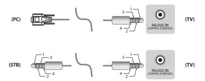
• You need to purchase the phone-jack to RS-232C cable required for the connection between the PC and the TV, which is specified in the manual.
