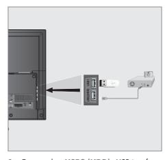
Connect the »USB2 (HDD)« USB interface on the television and the related data output on the external device (external hard disk, digital camera, card reader or MP3 player) with a USB cable;
