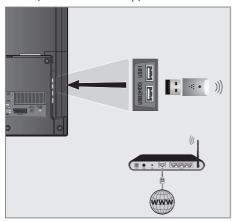
Connect Grundig WiFi USB dongle 2 to the »USB1« or »USB2 (HDD)« socket of your television in order to connect the television to a wireless network.
